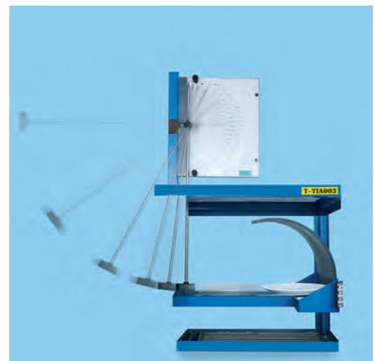
Mechanical resistance measured on a pendulum according to the EN 12980 standard of materials routinely found on the market:
